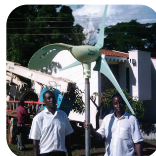
Small wind turbine weighing only 20kg Source : Zephyr Corporation
